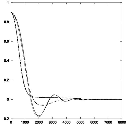
Fig. 5. Recovering solitary traveling solution  $u(z)=u(x+ct)$  of Eqs.(2), illustrating damped oscillatory ( $v^{-1} = 13.5, 14.5$ ) and monotonic recovery ( $v^{-1} = 20.0, 50.0$ ).
