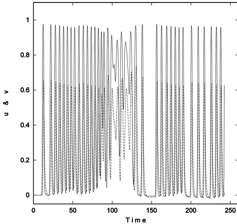
Fig. 4 Time variation of the excitatory and the recovery variable recorded in the medium at the location (10,10). The dotted one is the variation of  $v$ .
