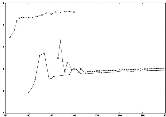
Fig. 6. Dispersion curve: Instantaneous wave speed as a function of period for  $v^{-1} = 13.5, 14.5, 50.0$  respectively from bottom to top, computed by repetitively stimulating at one of the ends of an open line.
