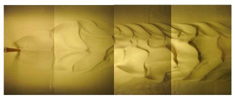
Fig. 4. Sedimentary structures downstream the cylinder; Re=42000 (Test 2)
