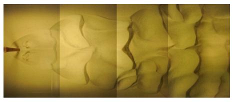
Fig. 5. Sedimentary structures downstream the cylinder; Re=43000 (Test 3)
