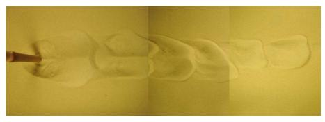
Fig. 3. Sedimentary structures downstream the cylinder; Re=38000 (Test 1)
