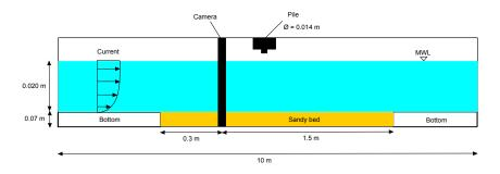
Fig. 1. Sketch of the experimental setup
