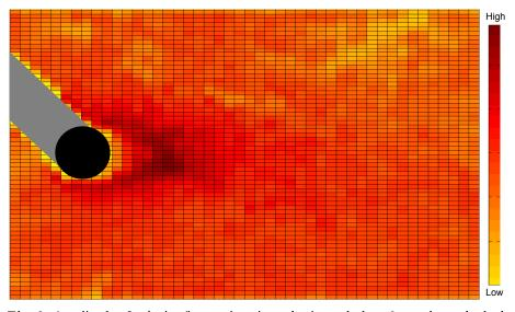
Fig. 6. Amplitude of velocity fluctuations in an horizontal plane 2 cm above the bed (Re=42000)
