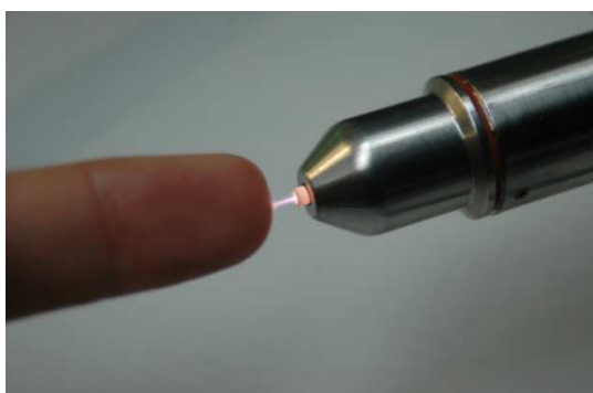
Figure 1: Photograph of the kINPen Med® plasma interacting with a fingertip.
